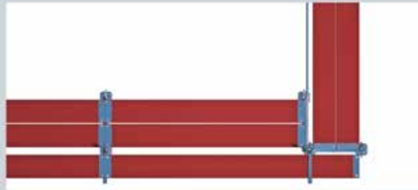
Clever – Gaps resulting from cornered structures are closed by applying correspondingly longer scaffold planks. Decks are then reliably secured against lift and slip.
